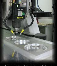
A massive aluminum plate is being loaded on one of YG Acoustics<sup>TM</sup> CNC machines, custom-made by Portatec in Germany.
